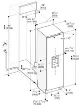
The maximum door front dimensions are based on a clearance of 3emm
